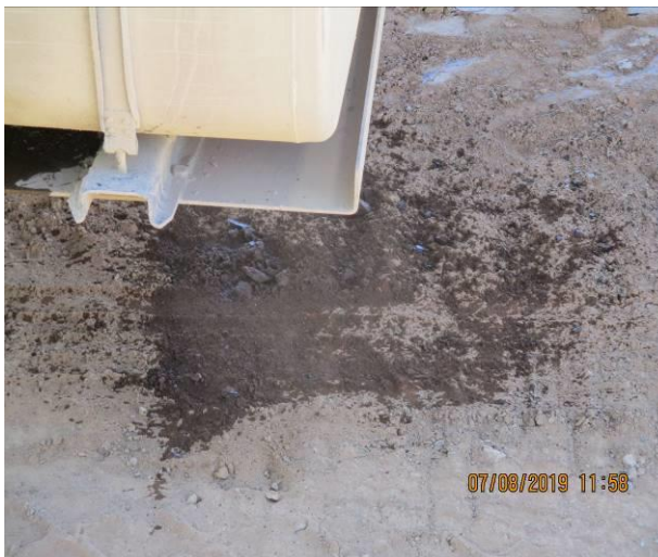
Photo: Diesel spill at refuelling area.
