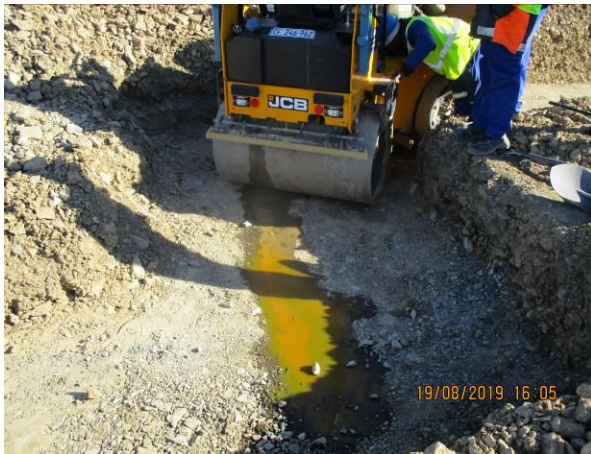
Photo: Hydraulic pipe burst from bomag roller. Photo: cleaning in progress.
