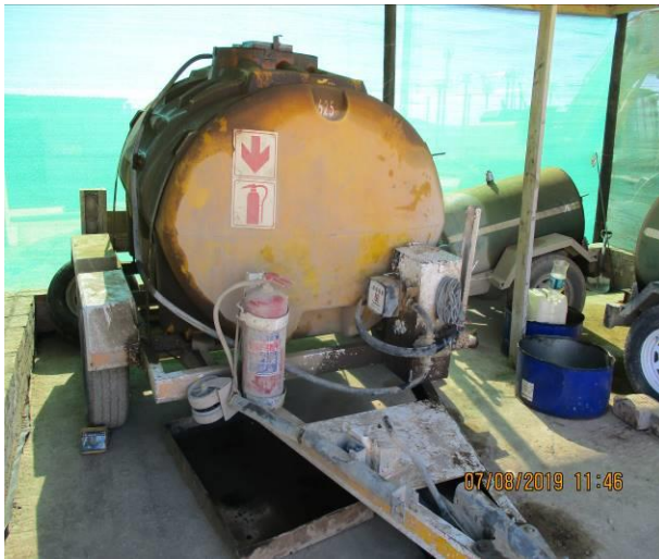
Photos: Leaking diesel bowsers.
